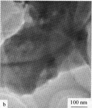
Fig. 4 TEM of textures of (a) cured PN-PAA and (b) carbonized PN-PAA
